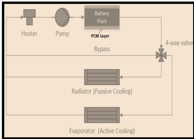
Figure 4: The combined liquid system with PCM system
