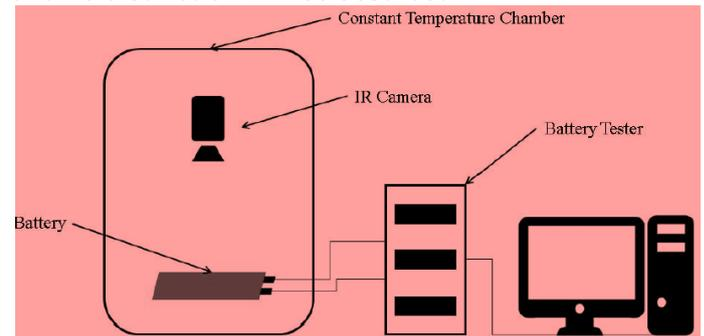
Figure 5: Schematic of the experimental setup
